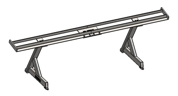
1. Assemble two parts (1) with part (2). Use eight countersinked screws M10x25 and nuts M10.
